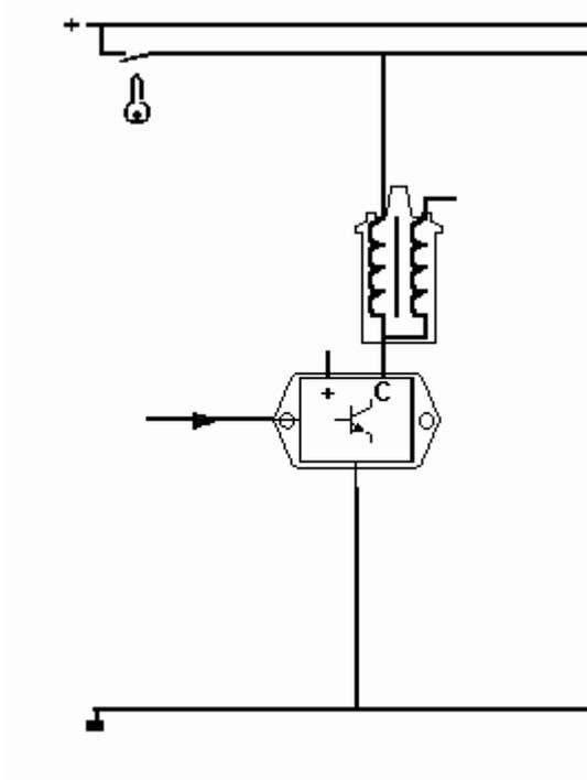
A current through the primary coil induces a magnetic field. The moment the current is switched off, the magnetic field suddenly disappears. This change of magnetic field induces an induction voltage and causes a spark.
