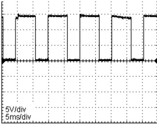
The control unit controls the current through the coil switching the current on and off with a certain duty cycle. The current increases as the duty-cycle increases. The duty cycle varies between approx. 35% (valve closed) and 85% (valve opened). Nominal idle speed is obtained when slightly open.
