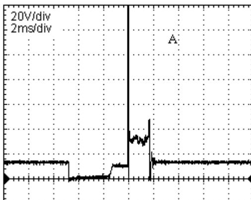
The oscilloscope images A and B gives you an example of the primary voltage measured on two different current limiting circuits.
